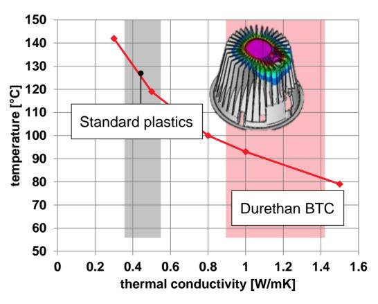
Exemplary temperature reduction depending on thermal conductivity
