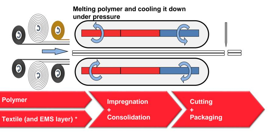
\*EMS layer: Metal mesh (Cu, steel), metal film (Al, Cu, MuMetal), carbon fleece or shielding fleece
